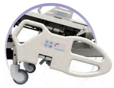
Siderail Controls , inner control allowing patient operates back, knee, Hi-Lo & auto-contour functions; and outer control provides reading of backrest angle & prevent infection.
